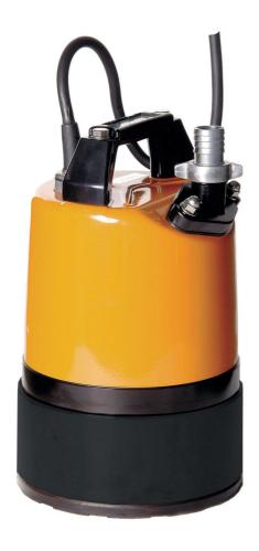
The LSC1.4S or "puddle sucker" is able to pump water down to 1mm, which makes it suitable for pumping large or small areas of nuisance water found on flat surfaces. It incorporates a dual position outlet port, to enable the user to position the outlet hose horizontally or vertically and avoid it kinking.
